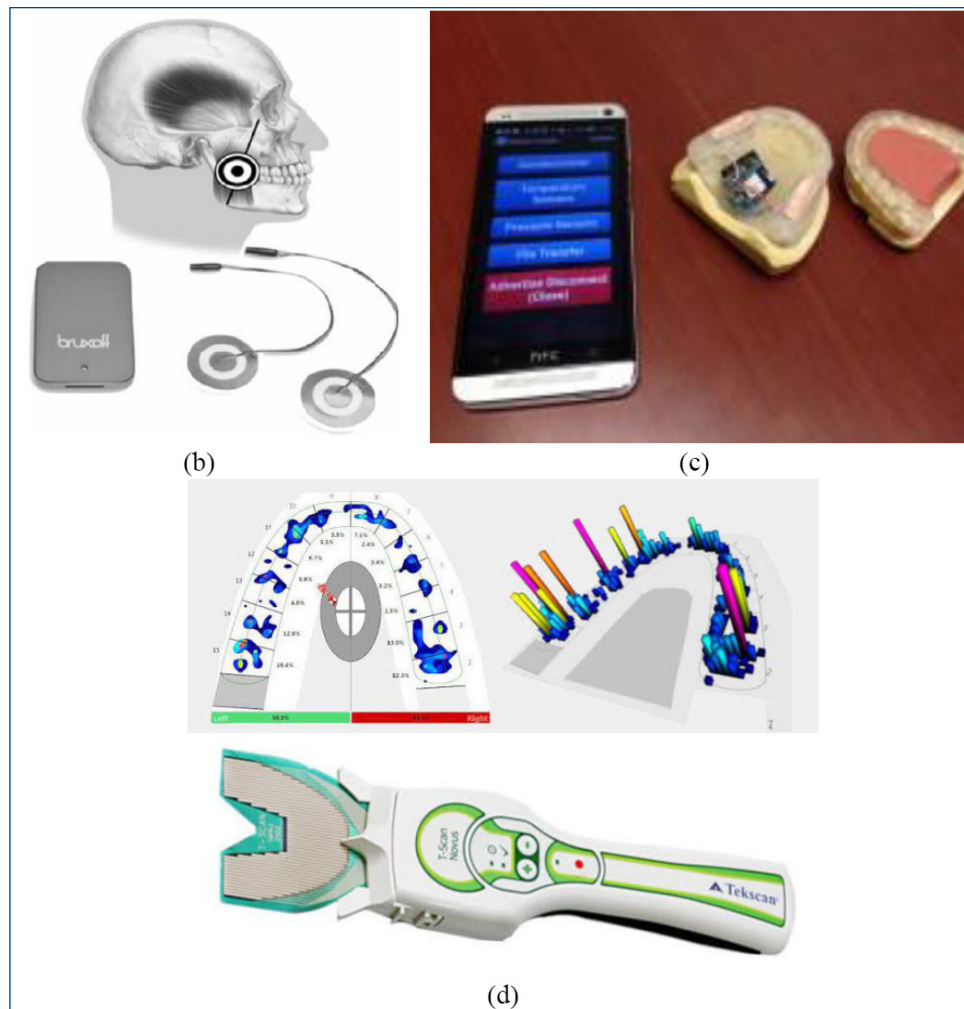
Figure 4. (a) Intra-splint force detector (ISFD) (b) EMG-EKG electromyography (c) Smart mouth guard (d) T-scan
